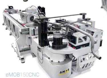
CNC tube bending machine
